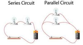
**Parallel Circuits** The loads placed along separate pathways. If one component fails the flow of electrons will continue on the other path.
