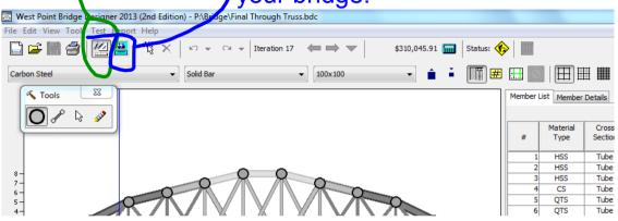
There are two ways to switch between Drawing Board and Load Test. There are two icons just below the test menu that allow you to switch screens. Or you can use the test menu to access the different screens.
